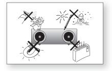
Protect the product from moisture (i.e. vases) , and excess heat (e.g.fireplaces) or equipment creating strong magnetic or electric fields Disconnect the power cable from the AC supply if the unit malfunctions. Your product is not intended for industrial use. This product is for personal use only.
